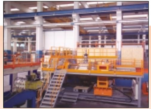
At Valvitalia's headquarters in Rivanazzano, major investments have been made into high-tech equipment. Shown is the assembly area, a welding facility for valves up to 60" in diameter and the massive test bench, believed to be one of the largest in the world.
