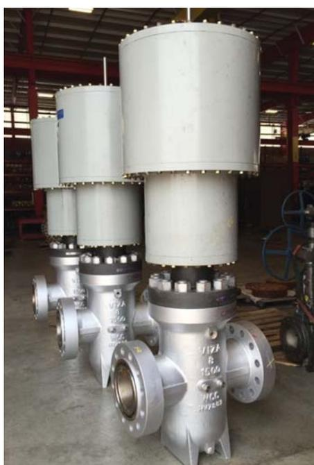
*API 6D through conduit slab gate valve*
