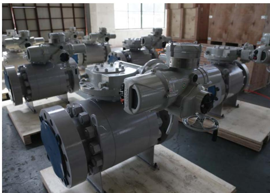
*Motor actuated metal seated ball valve*
