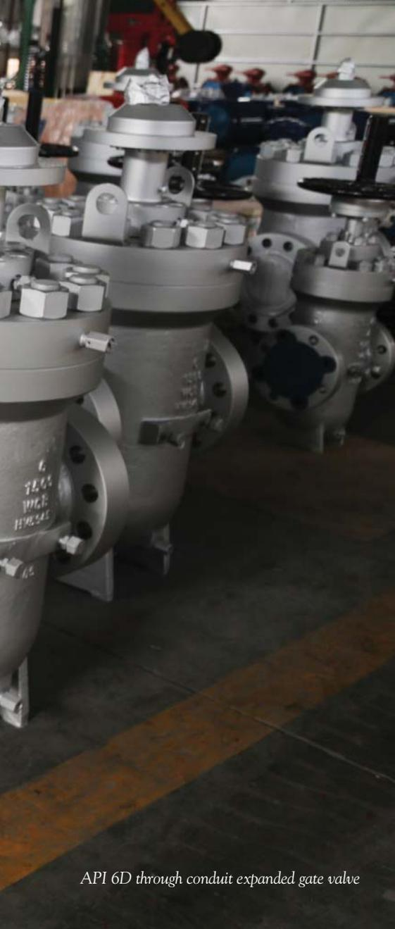
*API 6D through conduit expanded gate valve*
