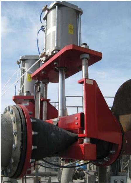
*The pinch valve in pneumatic conveying.*
