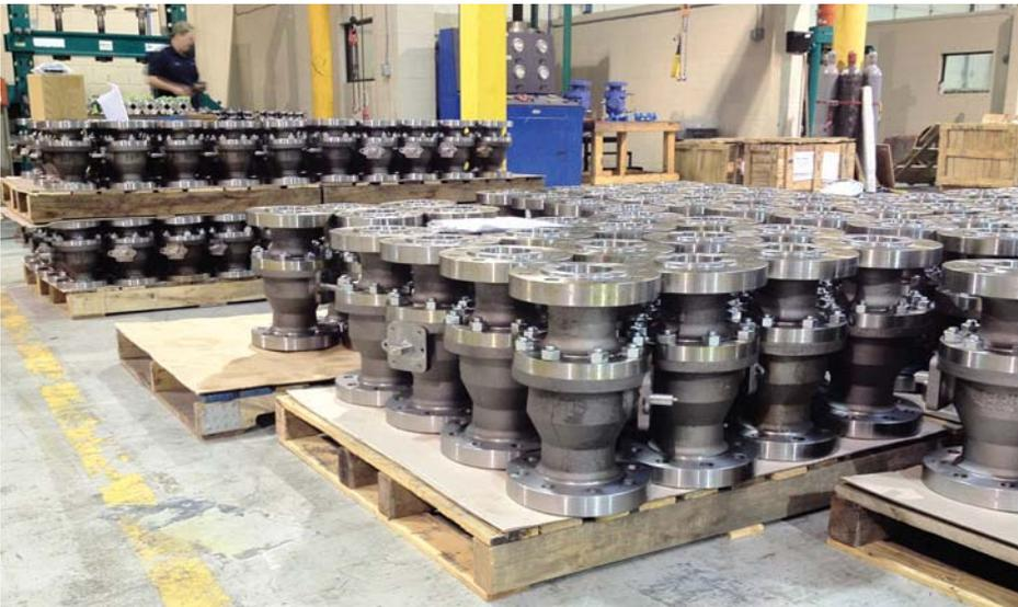
*ViNtrol Valves staged for Hydro Test.*
