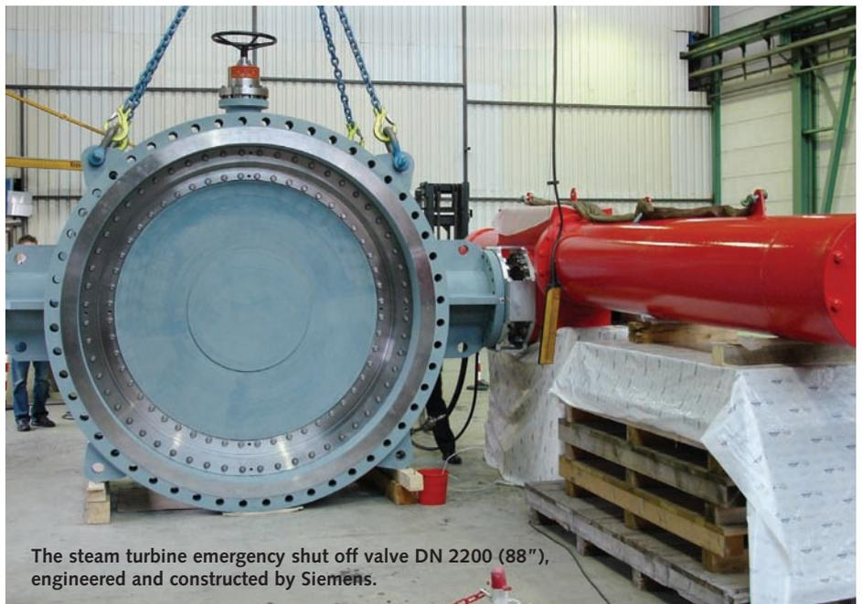
The steam turbine emergency shut off valve DN 2200 (88"), engineered and constructed by Siemens.
