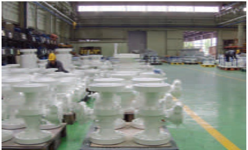
The final inspection area before the valves are crated and sent off to customers.
