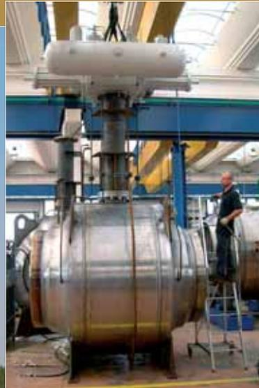
A 56" - 600# welded body under final assembly.
