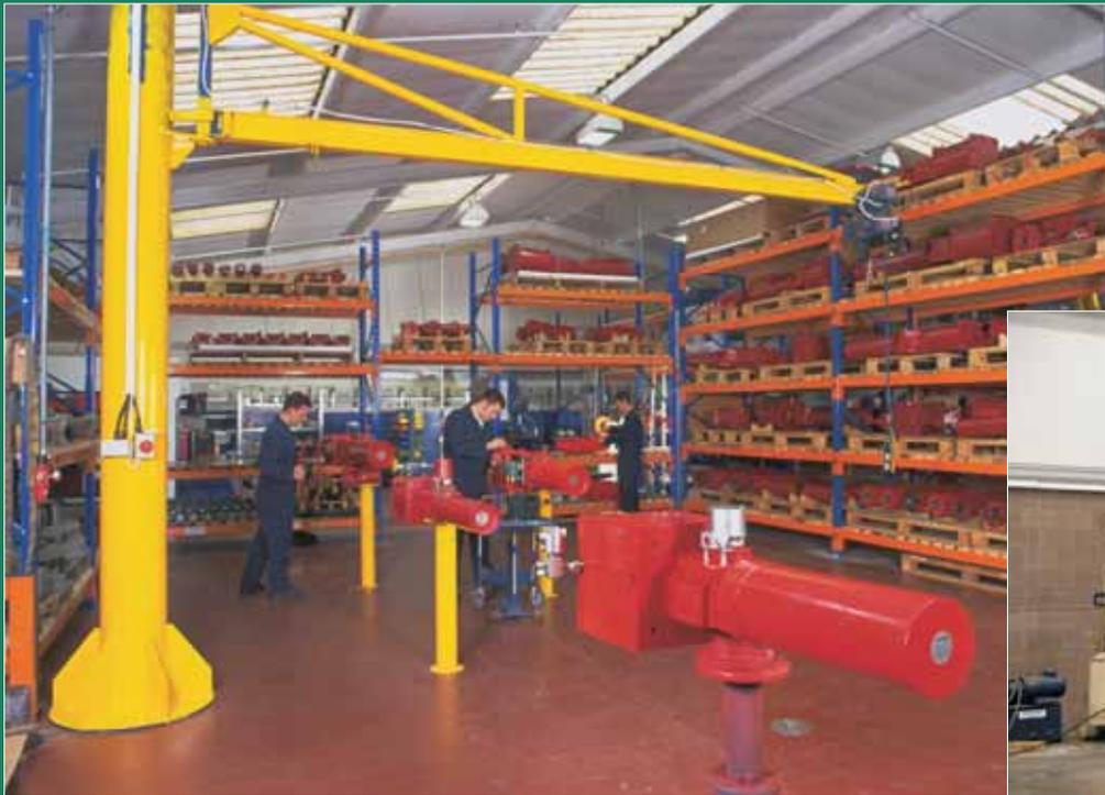
Actuator to valve assembly at the Calgary Centre of Excellence.
