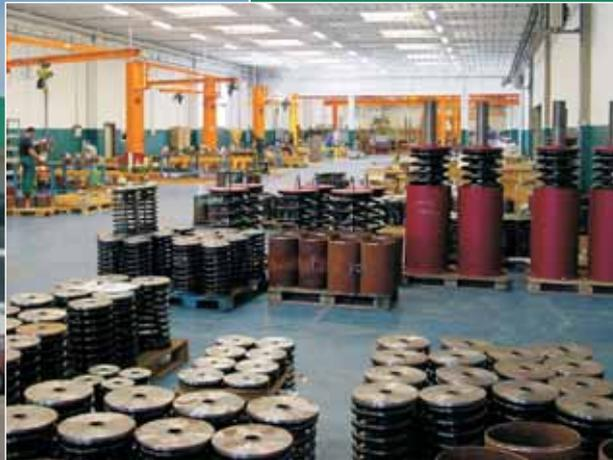
Pre-compressed spring packs for 1/4 turn and linear operators.
