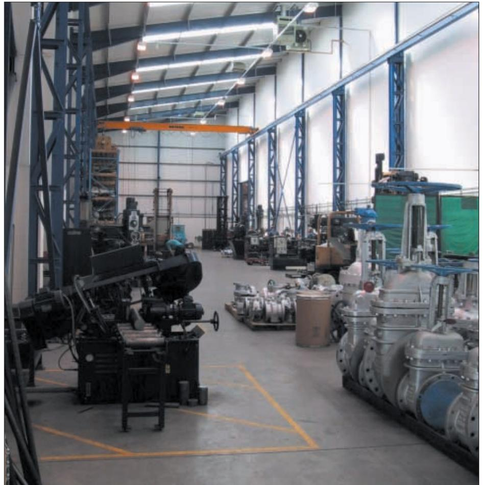
Most Transmark locations benefit from their own machine modification shops, where valves and actuators can be coupled to create complete flow control systems.
