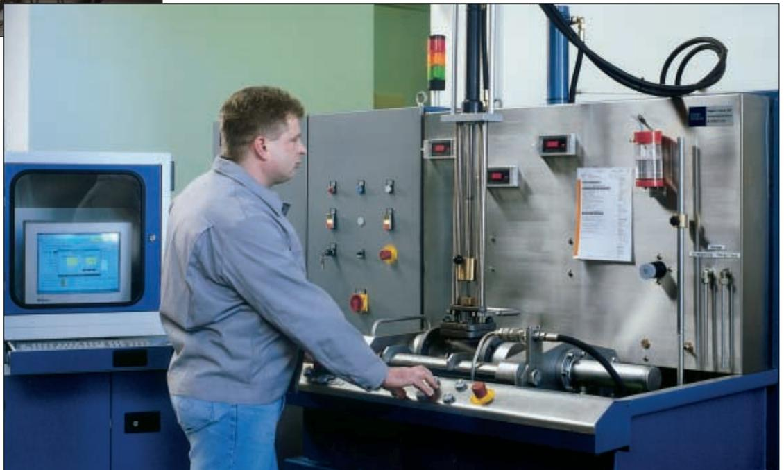
RTK fully tests all valves before they are allowed to leave the premises. Testing includes checking the seat tightness; a key area all too often overlooked.
