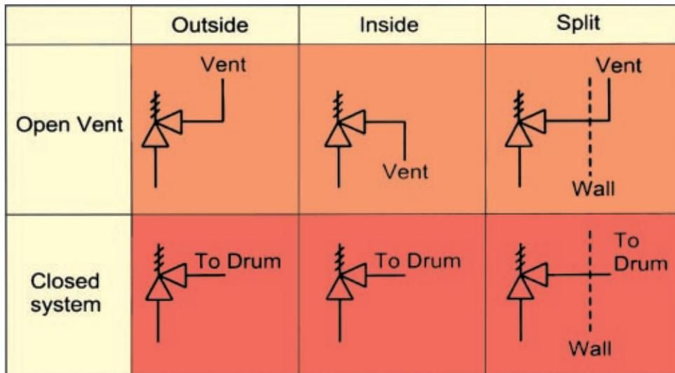
Figure 3. "Closed Systems" and "Open Vent" systems at a factory.
