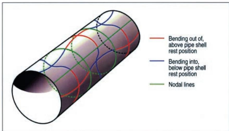
Figure 1B Standing waves on a shell (formed by a pipe wall)
