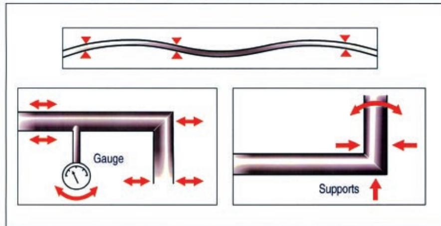
Figure 1A Whole body modes of vibration (partially supported pipe systems)
