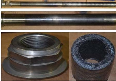
product line endured the demanding nature of the testing. As seen in the picture above, minimal to no wear was observed on the stem thread or its corresponding bushing.
