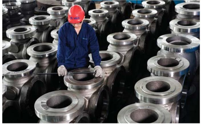
decided to acquire Jiangsu Taibo Casting back in 2010. With a single casting capacity of 3000 kg and annual production capacity of 6,000 tons, the foundry is capable of casting various material combinations: carbon steel, alloy steel, stainless steel, duplex stainless steel, etc.
