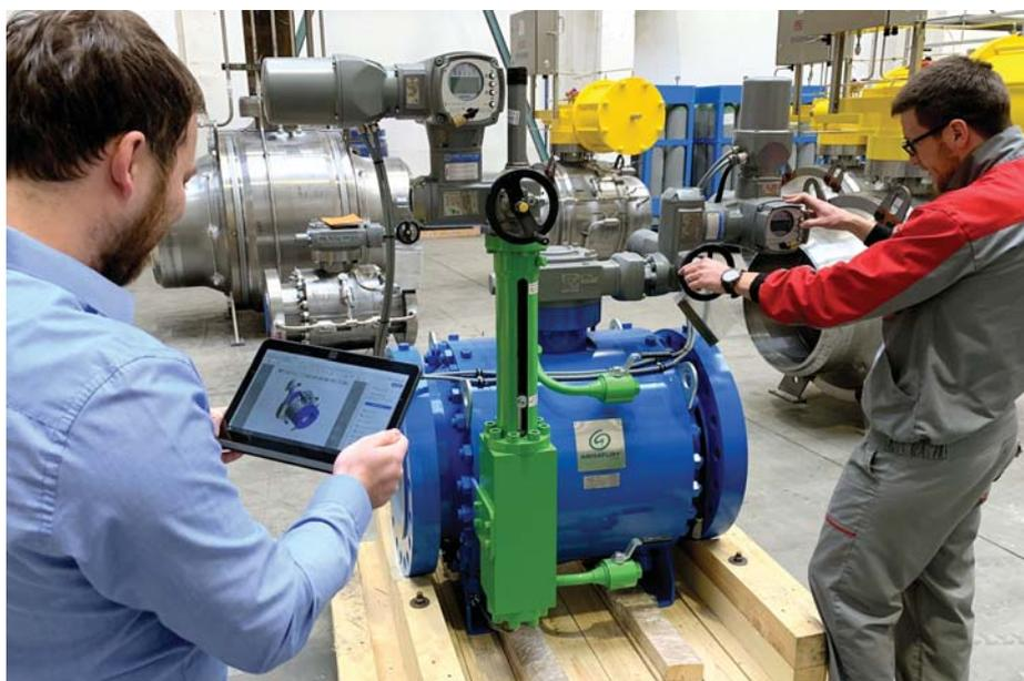
Part of the R&D-team testing prototype ball valve with retractable seats.
