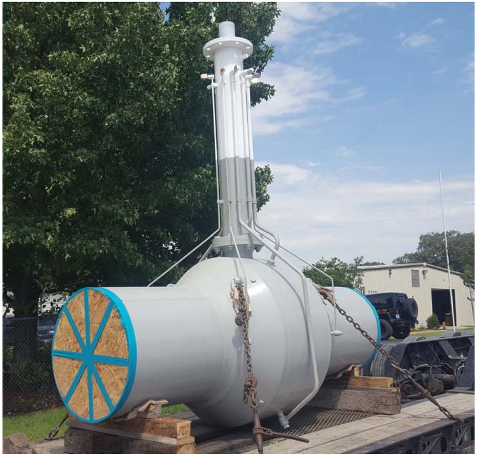
CIRCOR | KF Valves Welded Body Valve
