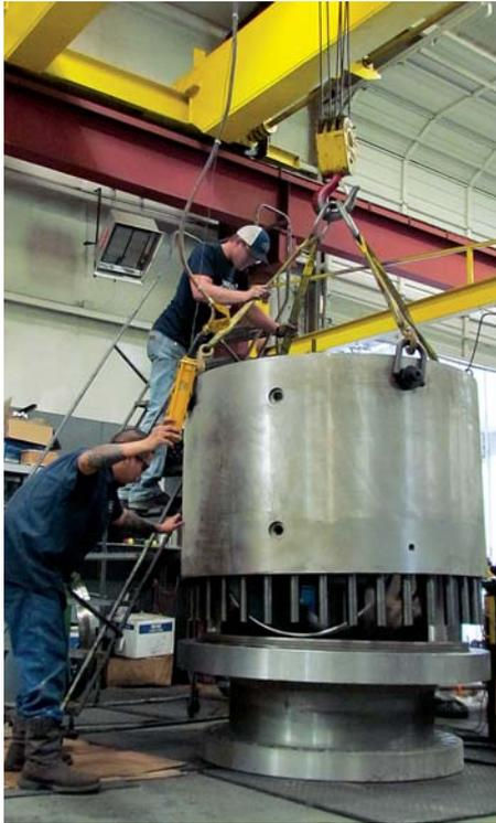
*Assembling 36” 600 SCV Trunnion Mounted Ball Valve.*
