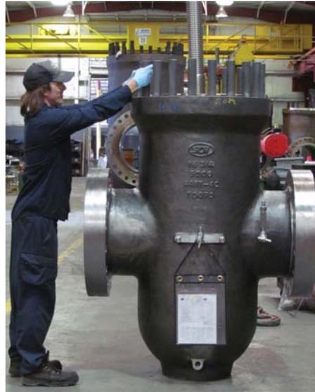
Assembly of 16-3/4" – 5000 PSI SCV API 6A Thru Conduit Gate Valve (Expanding Gate Design).
