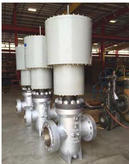
*API6D through conduit slab gate valve.*
