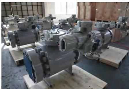
*Motor actuated metal seated ball valve.*
