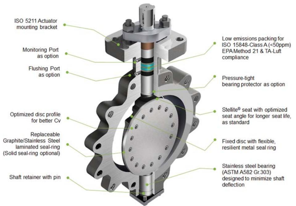
or binding of the disc, and lower the operating torque, the new valve can reduce total cost of ownership by up to 50%," he said. "Additionally, a precision machined metal seat and seal ring deliver reliable and bi-directional shutoff in high-temperature, high-pressure and severe service applications among others. The right-angle conical design facilitates frictionless in-line sealing."
