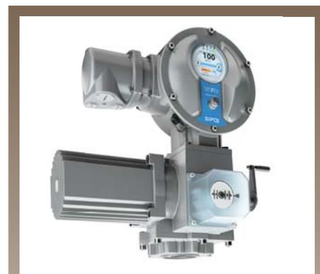
Specialised technology including an integrated frequency converter enables SIPOS to provide actuators with variable speed control. Soft-starts and finishes are facilitated, avoiding problems such as water hammer.
