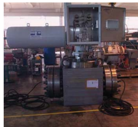
Forged 18" #1500 Top Entry H.I.P.P.S. - SIL III Ball Valve under performance test.
