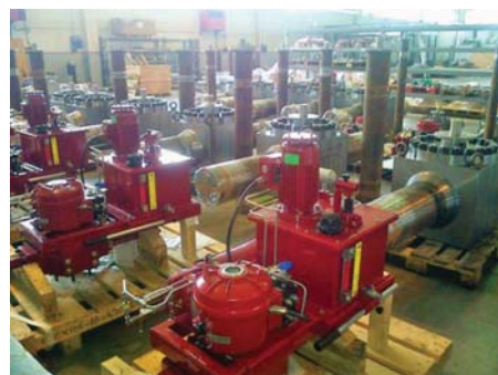
Electro-Hydraulic actuators and 12" #900 Top Entry Ball Valves.
