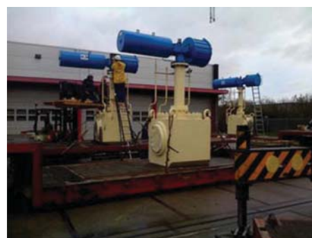
30" #1500 Forged Side Entry Ball V.
