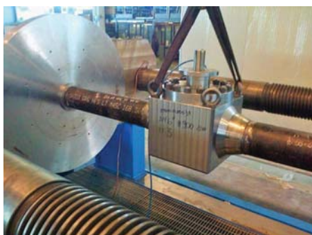
Forged Top Entry 6" #900 BW with pups under hydro-testing.
