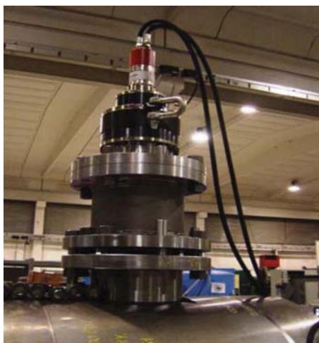
Torque test with Norbar torque tool with ca-pacity up to 100000 Nm.
