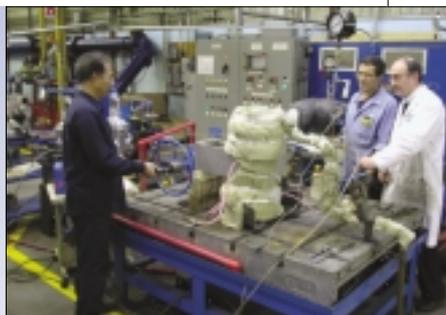
Velan's R&D team tests a metal-seated ball valve designed to meet a refinery's unique requirements.
