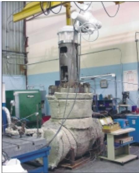
Diagnostic testing of a large gate valve at elevated temperature. This valve, destined for service in a nuclear power plant, is fitted with preinstalled thrust and torque sensors, signal conditioners and cabling (smart stems).
