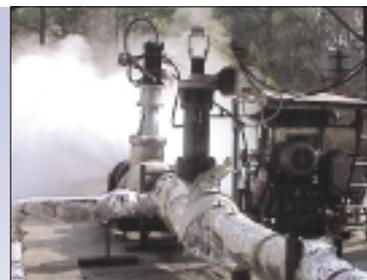
A loop isolation and blowdown test with hot pressurized water on a Velan 8" (200 mm) ASME Class 900 regular port isolation valve. Velan has been in the forefront of qualification testing for valves to address issues raised in the US Nuclear Regulatory Commission's Generic Letter 89-10.
