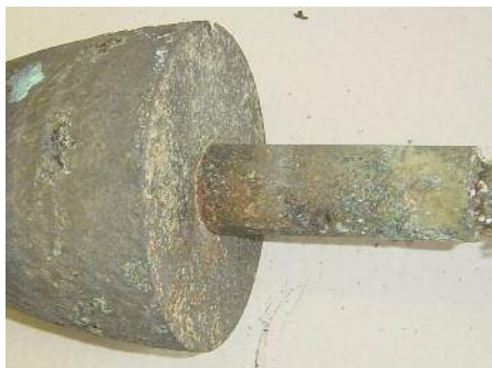
Fig. 1: Corrosion on a shaft of a valve
