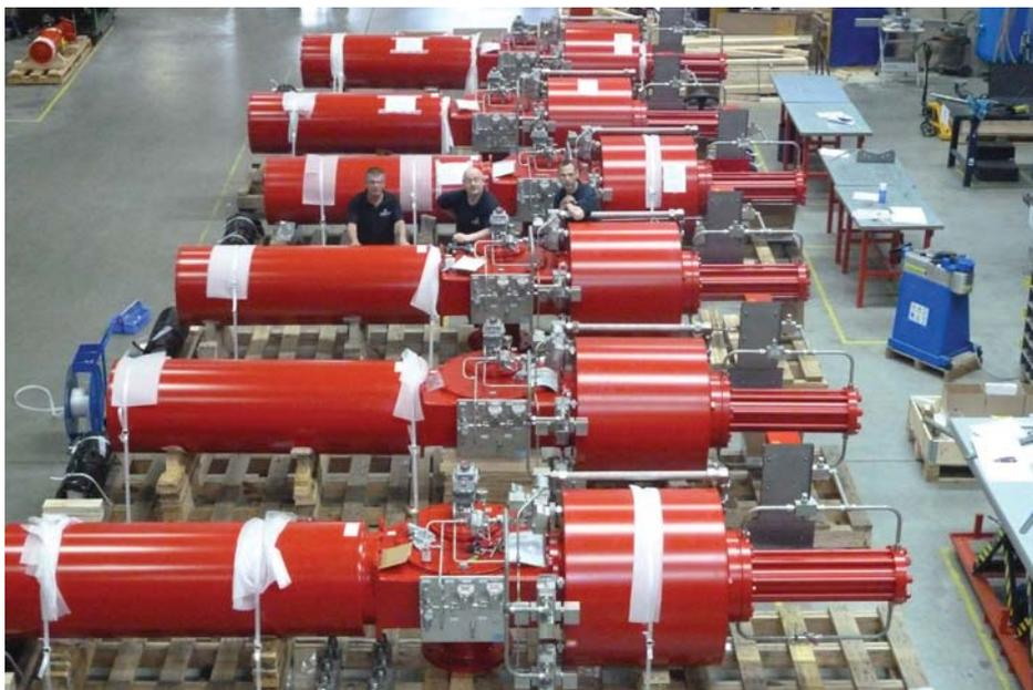
Some of the 16 actuators for HIPPS service are readied for shipment to, and installation on, a Western Australian offshore natural gas facility.
