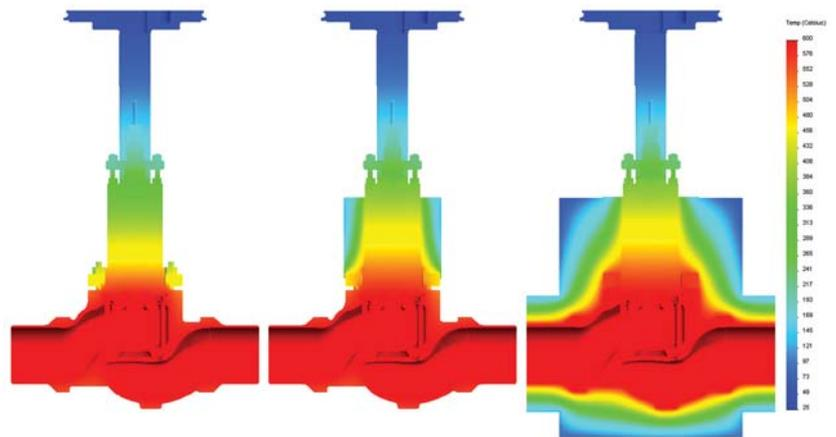
Figure 4: Temperature contours of non-insulated and insulated configuration of a 6" Mark One Control Valve with an extended bonnet.
