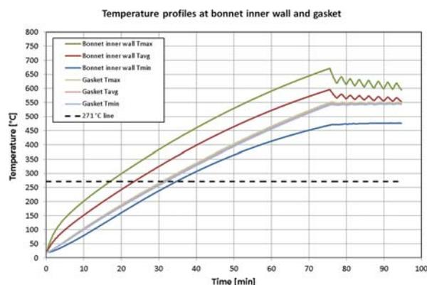
Figure 6: Temperature profiles of a 2" FlowTop Control Valve with a bellows seal bonnet at the bonnet inner wall and gasket during heating process from a cold start with heat tracers of 600 W around the bonnet outer wall and 1000 W around the valve body outer wall.
