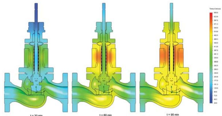
Figure 5: Temperature contours of a 2" FlowTop Control Valve with a bellows seal bonnet during heating process from a cold start with heat tracers of 600 W around the bonnet outer wall and 1000 W around the valve body outer wall.
