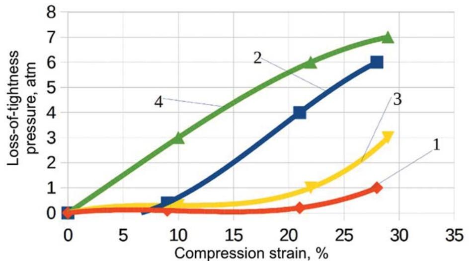
Figure 7. Air-tested joint tightness: a) test configuration; b) compression strain vs loss-of-tightness pressure for FRR with a cross-sectional diameter 5.8 mm and different core hardnesses (1, 2 — Shor A 55; 3, 4 — Shor A 70) and capsule thicknesses (1, 3 — 0.2 mm; 2, 4 — 0.7 mm).
