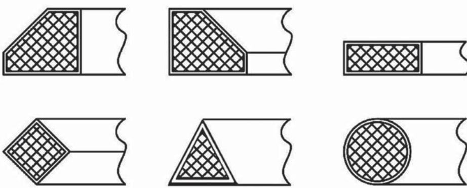
Figure 8. Cross-section configuration options for fluoropolymer-encapsulated sealing rings
