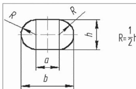
Figure 4. Contact area width calculation
