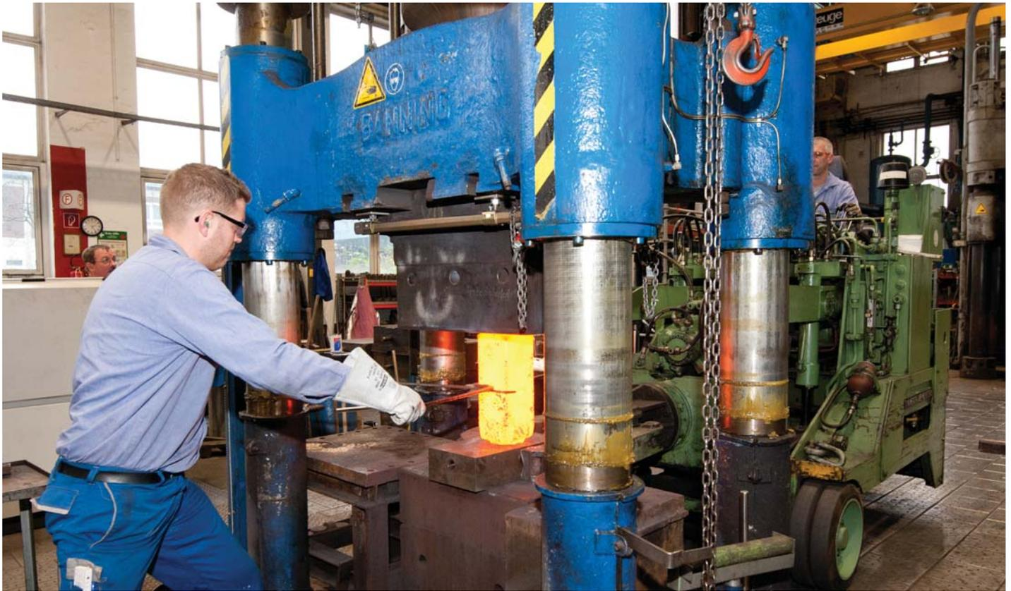
Forged stainless steel is a common material for BASF's high pressure valves. Courtesy BASF SE.
