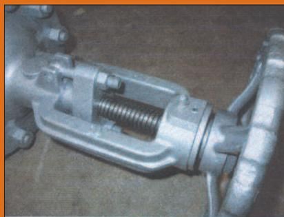
through out the 3500 cycles and the leakage rate for both was reduced to a single digit after re-setting the gland nut torque at cycle 3500. These independent tests were made in December 1999. These test results\* allowed us to guarantee a 50 ppm maximum VOC emissions leak rate for all "off the shelf" valves.
