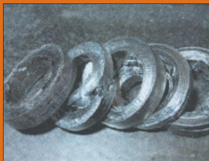
Fig. 1b: Packing rings after test.
