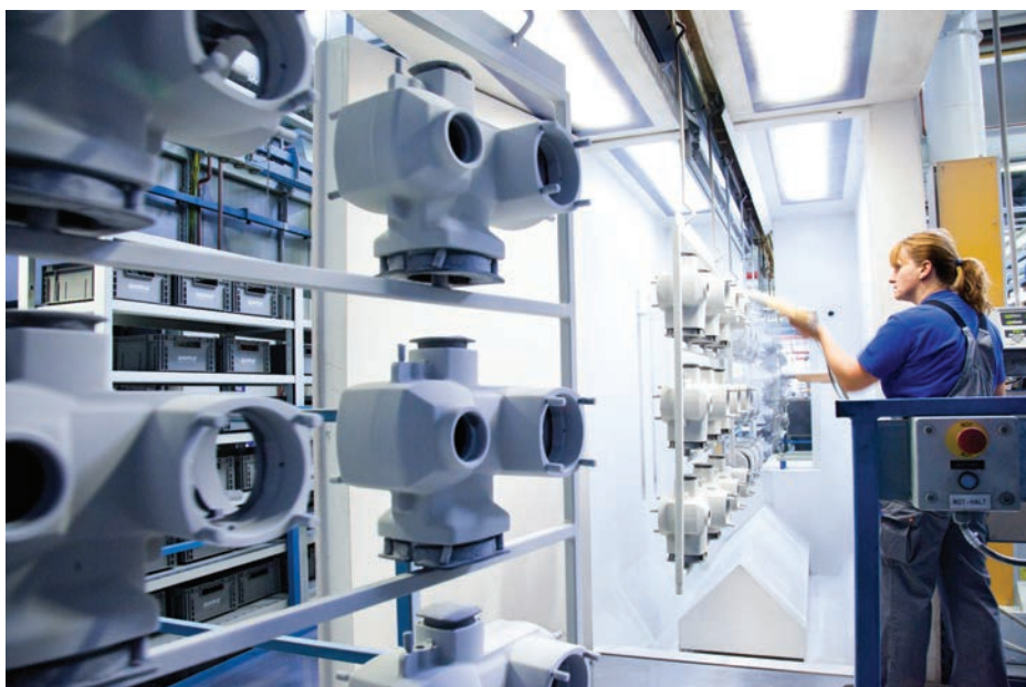
The recently completed, coating line which uses powder technology to guarantee a longer life of the product as well as protection from corrosion.
