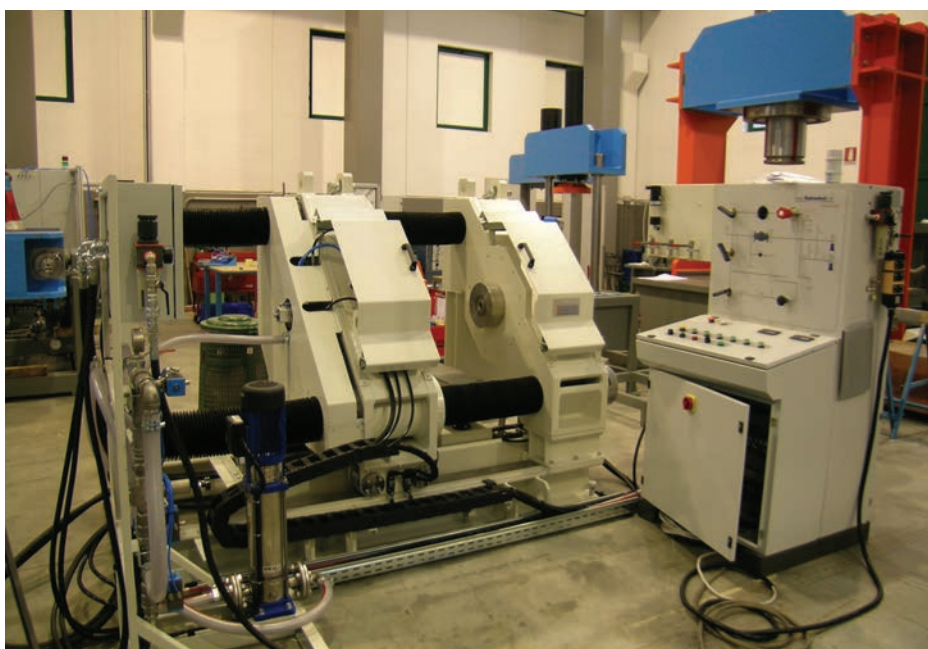
A 200 tons test unit for valves that are used in nuclear applications.
