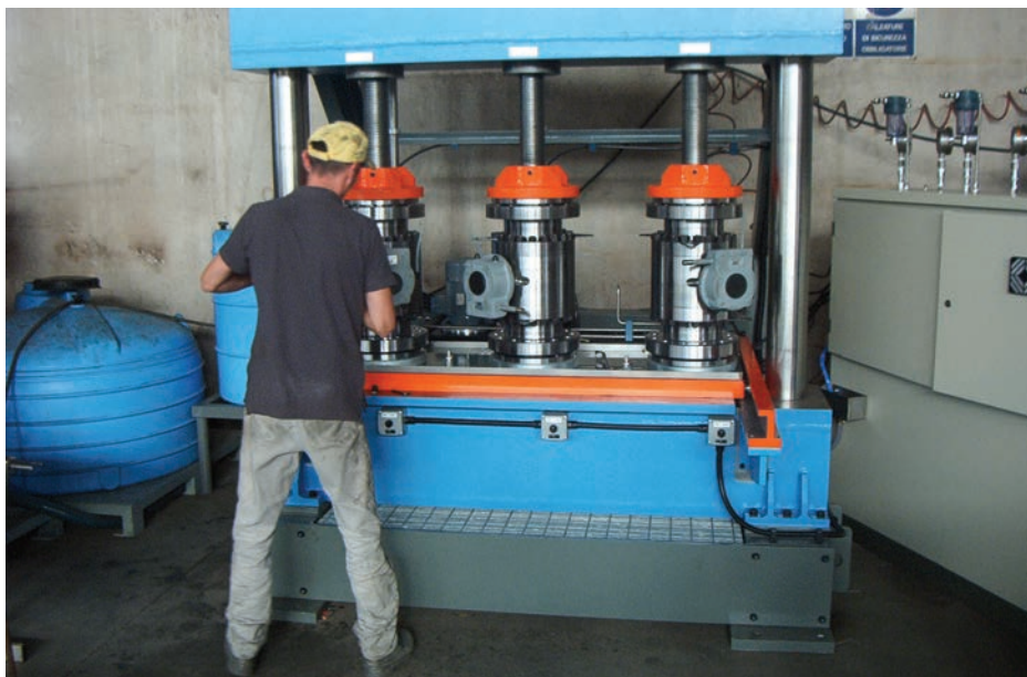
A multi-station vertical test unit which can test 3 times 120 tons.
