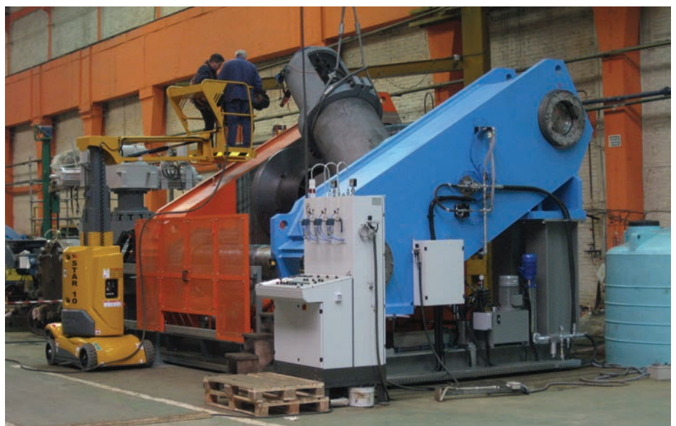
Italcontrol staff working on a horizontal test unit which is suitable for 5000 tons.
