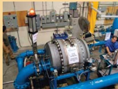
*Qualification testing of a 34" titanium triple-offset butterfly valve in Velan's R&D lab. The valve had no leakage over the 10,000 cycle test.*
