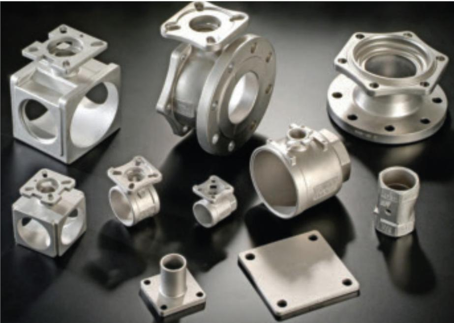
Haitima Corporation also produces singles parts of valves which are then exported to customers. This picture shows some castings in various sizes and the picture below shows some of the stainless steel balls which are also produced in the Zhongshan factory.
