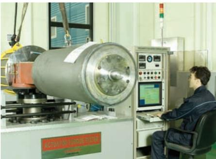
Flowbus has developed a unique digital torque tester which enables them to accurately measure an actuator's torque output.
