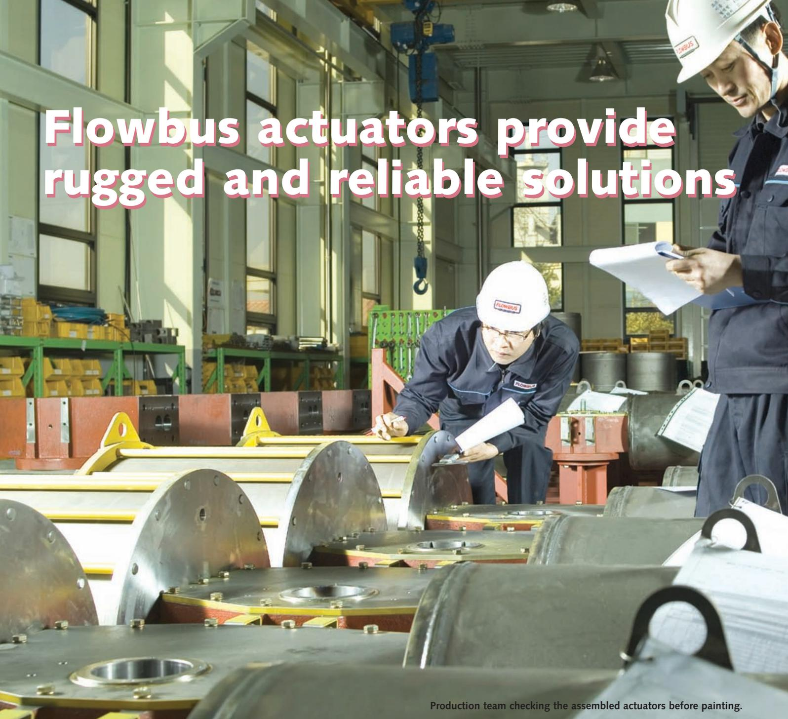
Production team checking the assembled actuators before painting.
