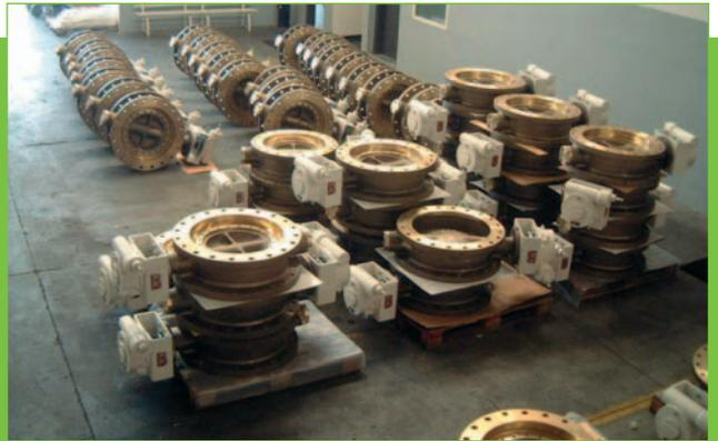
The MV is also ideal for ESDV applications. These valves, made of Monel and 316L, are used in oxygen and hydrogen plants at Sasol, South Africa.
