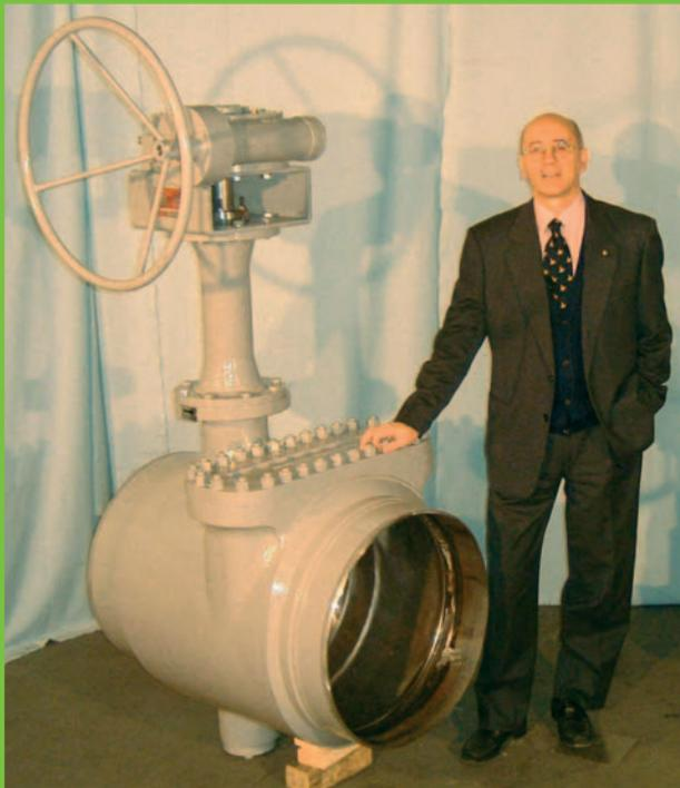
This DN 30", #600 cryogenic MV model was destined for the Damietta project in Egypt.
