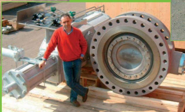
The MV valve can be used throughout the gas chain. This DN 48" (1200 mm) ANSI Class 300 model for modulating application was supplied through Snamprogetti for use in the Qatif Gas Plant in Saudi Arabia
