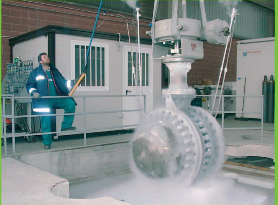
FCX Orton has invested in a massive bunker for cryogenic and high pressure gas test for valves up to DN 2600.
