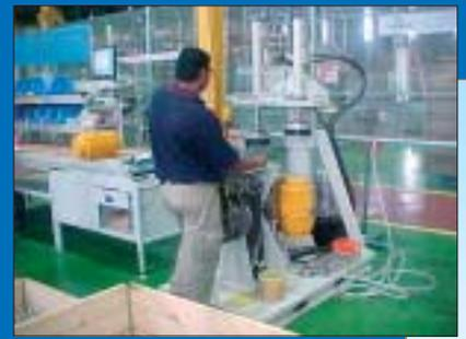
▲ The large LEAN assembly line spring press operation is used for El-O-Matic sizes E600 thru P4000 and Hytork size XL281 thru XL4586 actuators.
