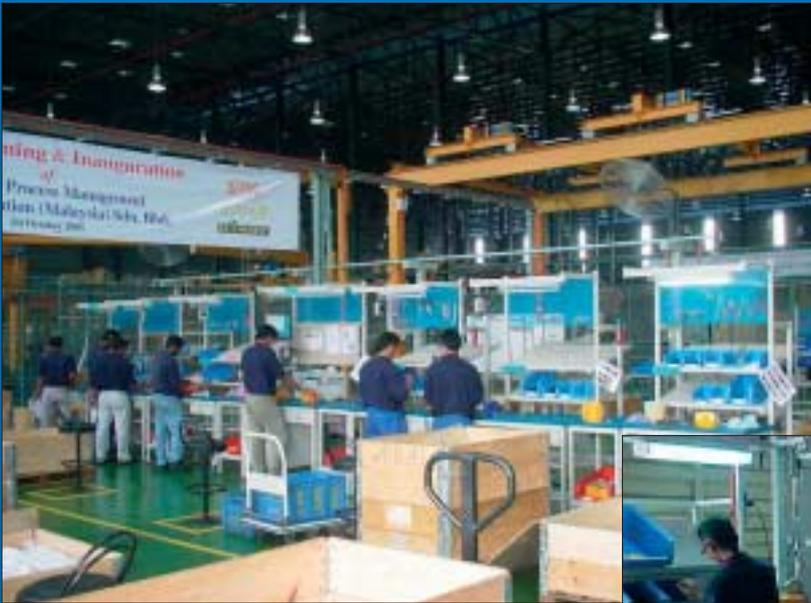
▲ One of the three Nilai LEAN assembly lines. This line produces the smaller El-O-Matic and Hytork products thru size E350 and XL221 actuators. All lines employ LEAN assembly techniques including three-bin KanBan and a seven stage progressive assembly approach.
