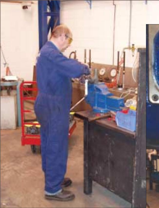
▲ Repacking a valve to prevent leakage.
