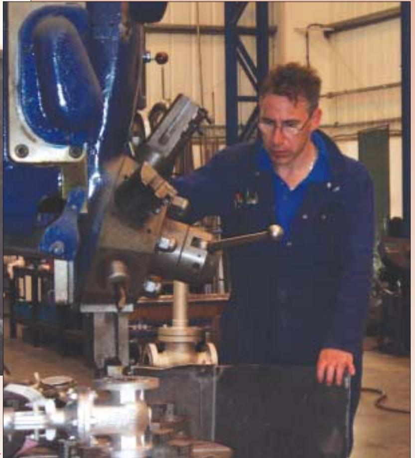
► Re-boring a valve to specific customer requirements.
