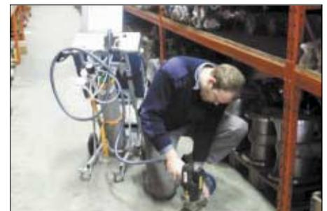
Investments in an in-house spectrometer enables chemical compositions and materials grades to be quickly checked.
