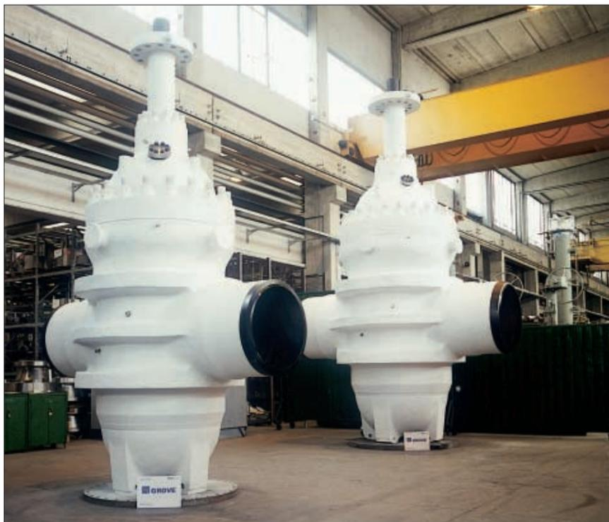
42" / 1500# G 12 metal seated gate valves used in the Statoil - Europipe II and Asgard project.
