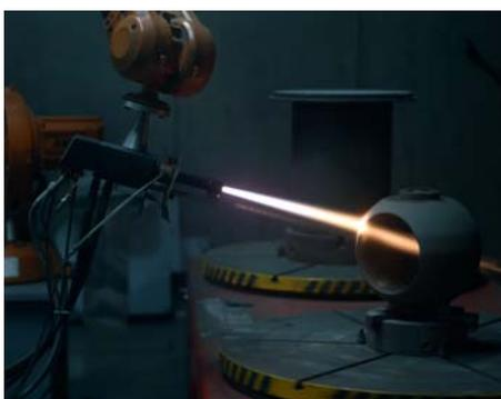
High velocity oxygen fuel spraying.
