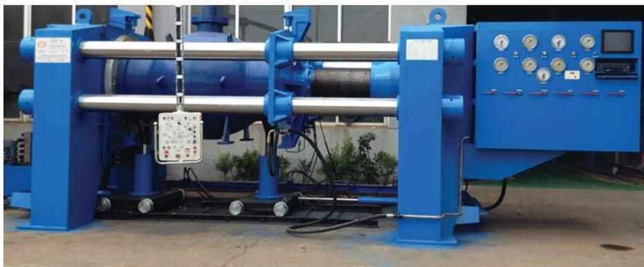
4600T super large screw top pressure valve test bench (Tianjin Cameron).
