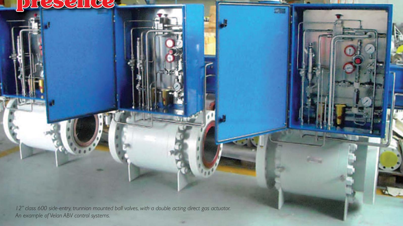
12" class 600 side-entry, trunnion mounted ball valves, with a double acting direct gas actuator. An example of Velan ABV control systems.
